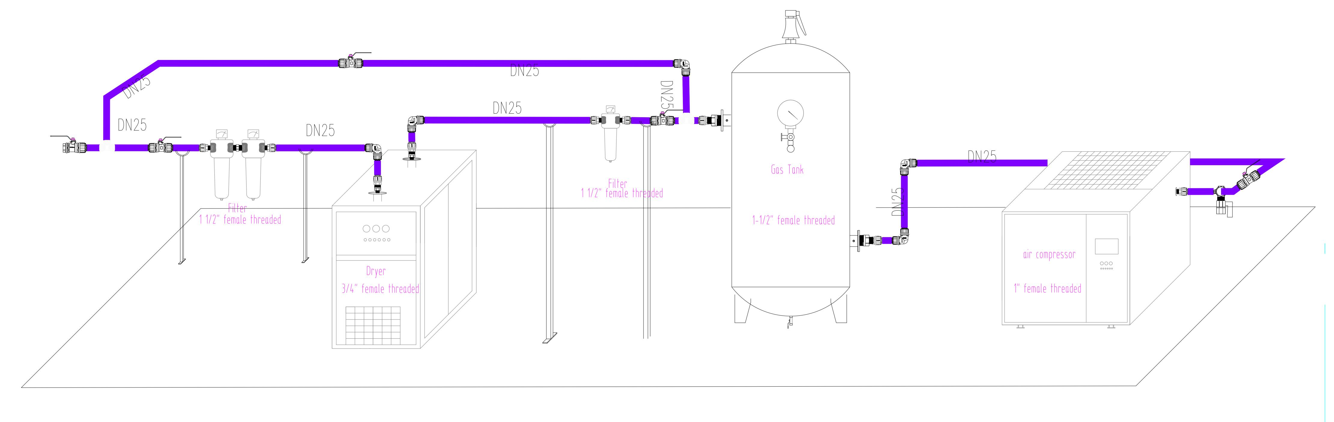
Compressed air pipeline layout drawing
